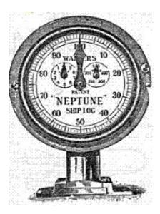
What the taffrail log actually measures is the number of revolutions of its finned rotor at the end of a log line as it is pulled through the water. Its accuracy in recording nautical miles depends on how well it was calibrated at different speeds, when it was calibrated last, and its overall condition, including the log line and all internal parts. So let us simply refer to the log readings that were given as "log-miles."
