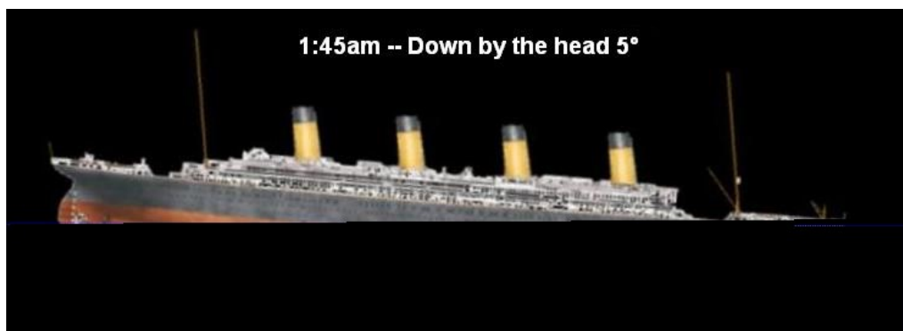
Fig. 3 – Titanic trimmed down by the head about 5^\circ .
