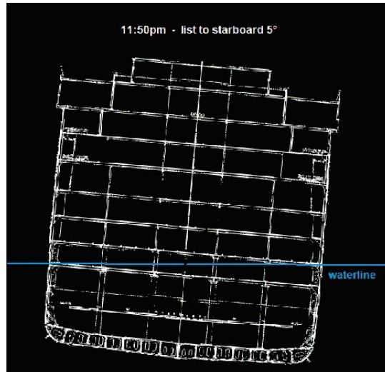
Fig. 1 – Cross section of Titanic looking forward with 5° list to starboard.
