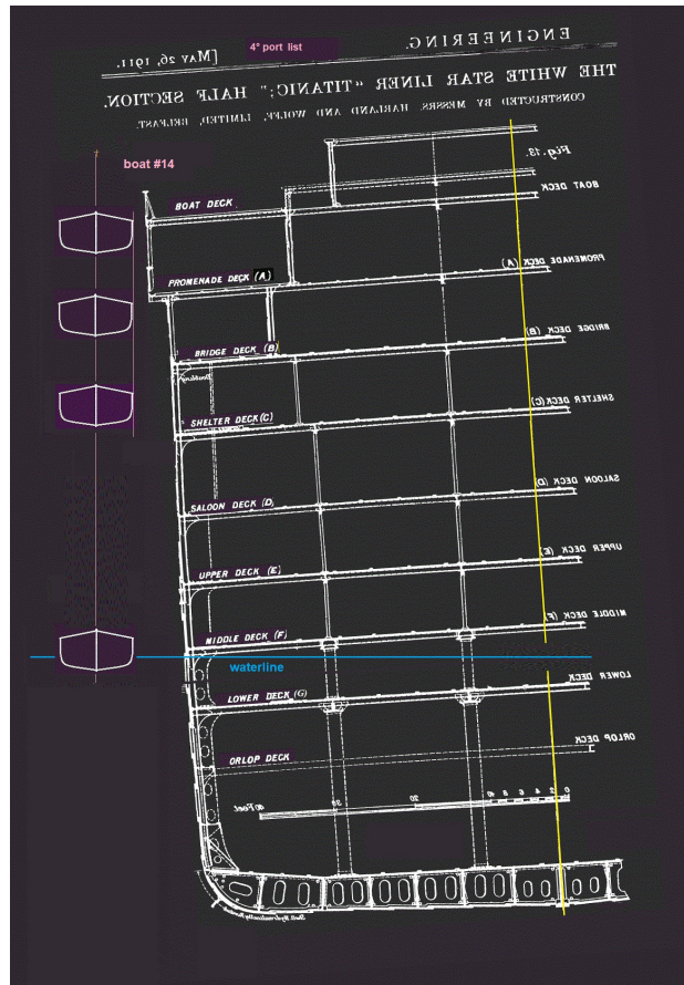
Fig. 20 – Half cross-section of Titanic showing a 4^\circ list to port in vicinity of boat No. 14 looking forward about 1:35am.
